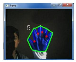
This is hand glove recognition system as virtual mouse for hci used for mouse operation with hand glove.
