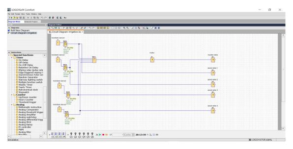
1) when moisture sensor 1 is initiated, master valve and zonal valve 1 gets open
