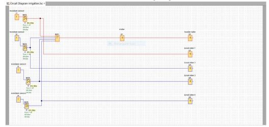
2) When moisture sensor 2 is initiated, master valve and zonal valve 2 gets open
