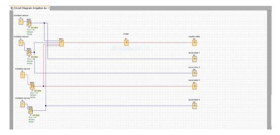
4) When moisture sensor 4 is initiated ,master valve and zonal valve 4 gets open
