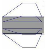
The fins are trapezoidal finset. Fins are used for better stability tilted at an angle of 22.5 degrees The fins are made of Carbon Fibre.
