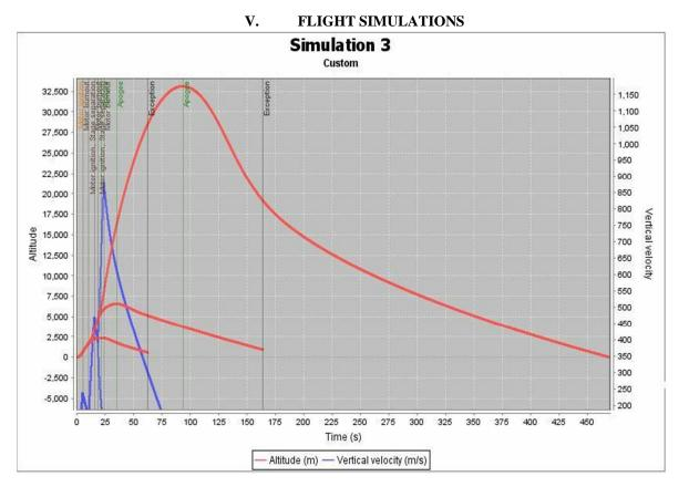
The Altitude and Vertical Velocity Is Plotted With Respect to Time. Different stages of flight are shown in the simulation graph. For example, Motor Burnout, stage separation etc. The launch rod length was set to1100cm (double the length of the rocket)
