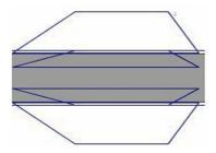
The fins are trapezoidal fin set. Fins are used for better stability tiltedatan angle of 22.5 degrees The fins are made of Carbon Fibr
