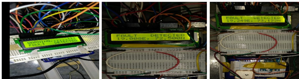
Fig. 10 LCD visual of "warning", "fault detected" and "location coordinates" after detection.
