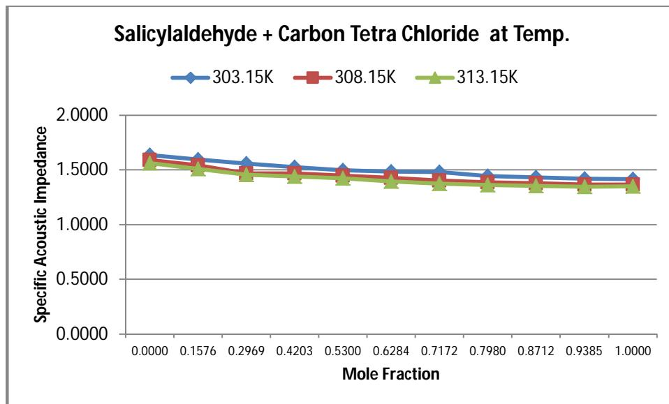
Specific Acoustic Impedance Vs. Mole Fraction
