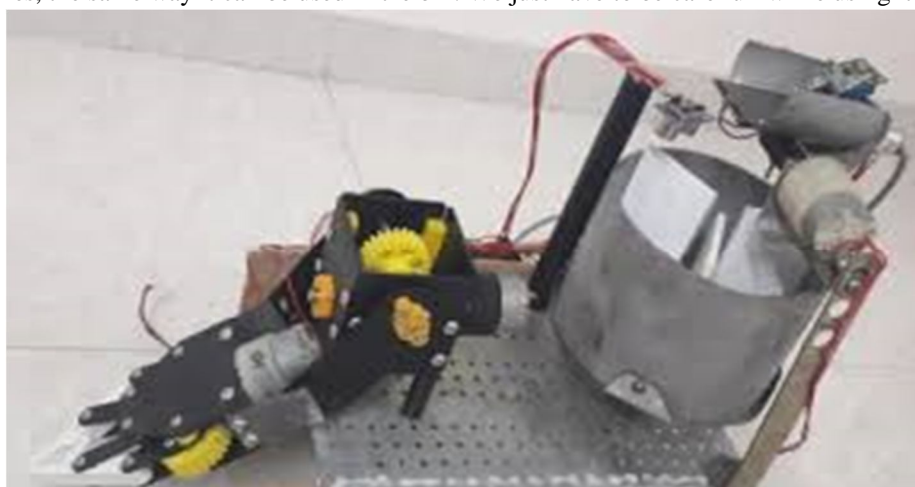
Fig 5. Robotic arm for segregation [20]
