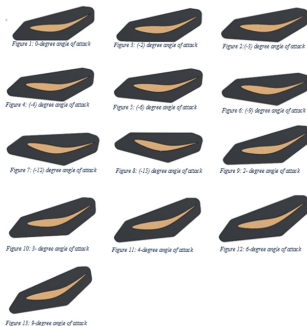
Fig. 3. Cross-Section of Spoiler at various angle of attack
