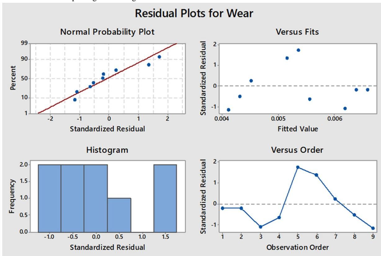
Figure 4: Residual Plots for Wear (mm<sup>3</sup>/min) V/s Load (N), Sliding speed (mm/s) of A357 alloy.
