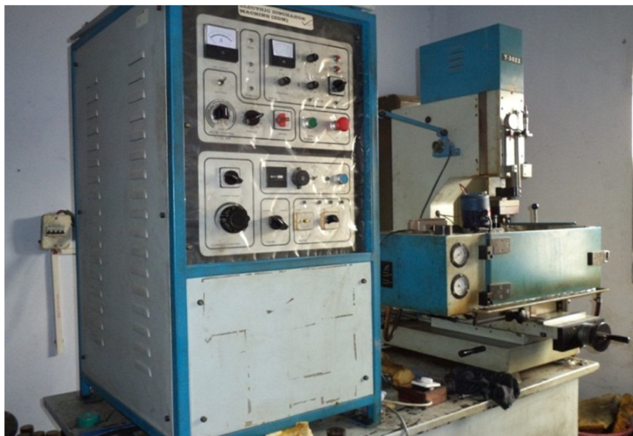
EDM machine with stirrer arrangement
