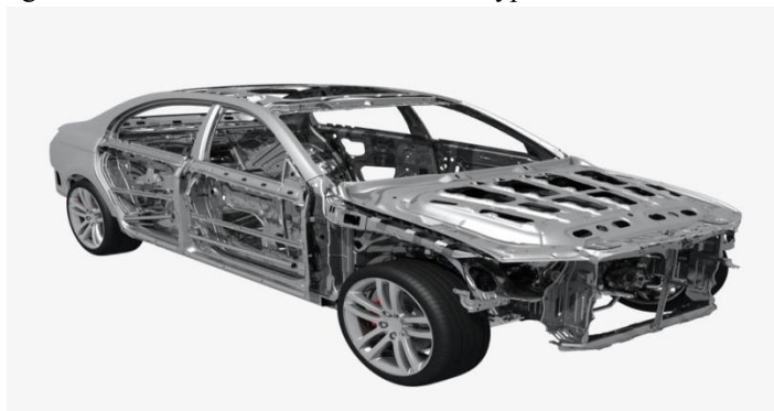
Figure 1. Semi-integral Chassis frame model
