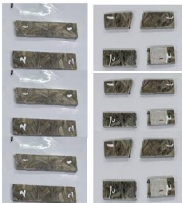
Fig 3.7: ILSS Testing specimen before and after test.
