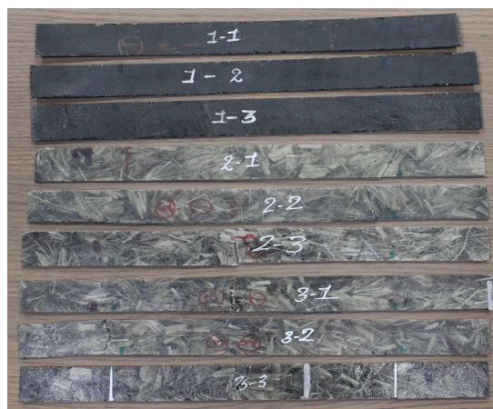
Fig 3.2: Tensile Test Specimens after test.
