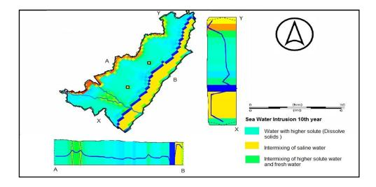
In this section, simulation has been done to predict the future scenario of the study area after 10 years and it shows the water intermixing is at peak with saline water because of higher extraction from a well and the colour composition is changed in comparison from 1st year and a study area has started yielding saline water.
