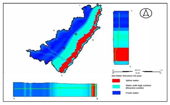
In this section, the scenario is set up in a way where the availability of freshwater can be seen whereas the extraction from the well was normal where no intrusion of saline or intermixing of saline water can be seen. The green line in AB section represents the water table.
