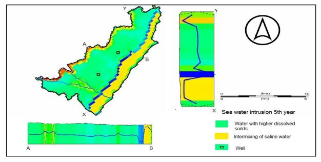
In this section, simulation has been done to predict the future scenario of the study area **after 5 years** and it shows the water intermixing has been started with saline water because of extraction from a well and higher presence of solute in the water which is coming out from the system because of higher density of the saline water.
