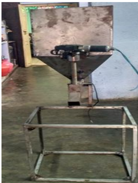
Fig 1: Fabrication of Smart Storage and Dispensing Machine for Food Grains
