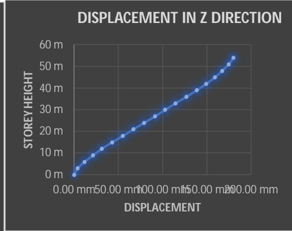
Figure 4b: Displacement in Z direction
