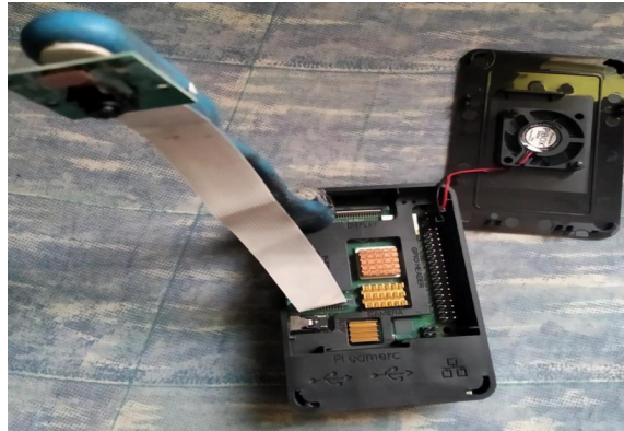
Fig.1. Connectivity of Camera with Raspberry Pi
