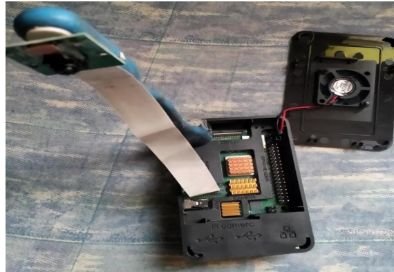
Fig.1. Connectivity of Camera with Raspberry Pi
