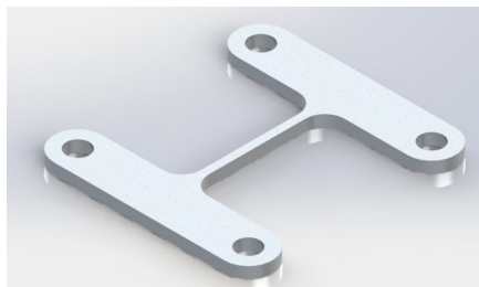
Fig. 27: CAD rendering of Aluminum busbar used to make series and parallel connections.
