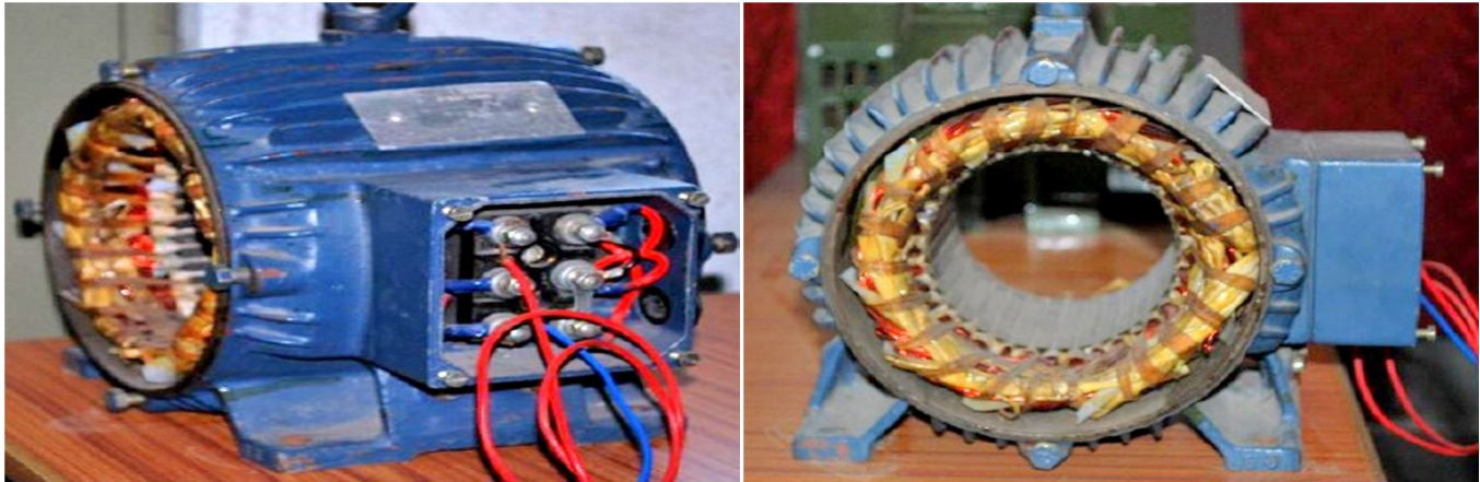
Figure 2: Wound stator of an induction motor
