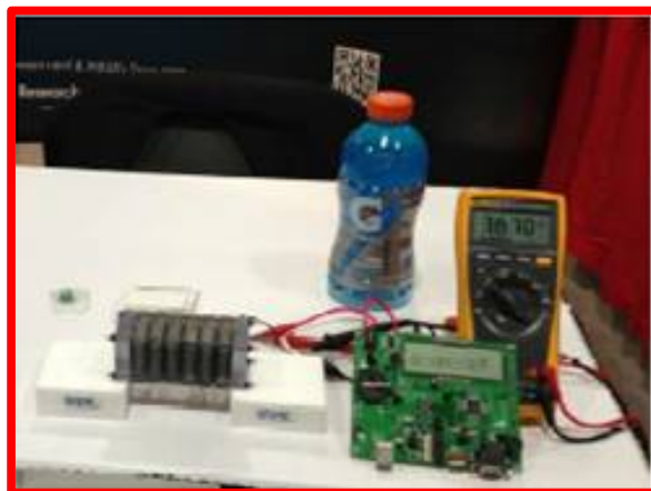
Fig(14)Microprocessor and LCD powered by bio battery
