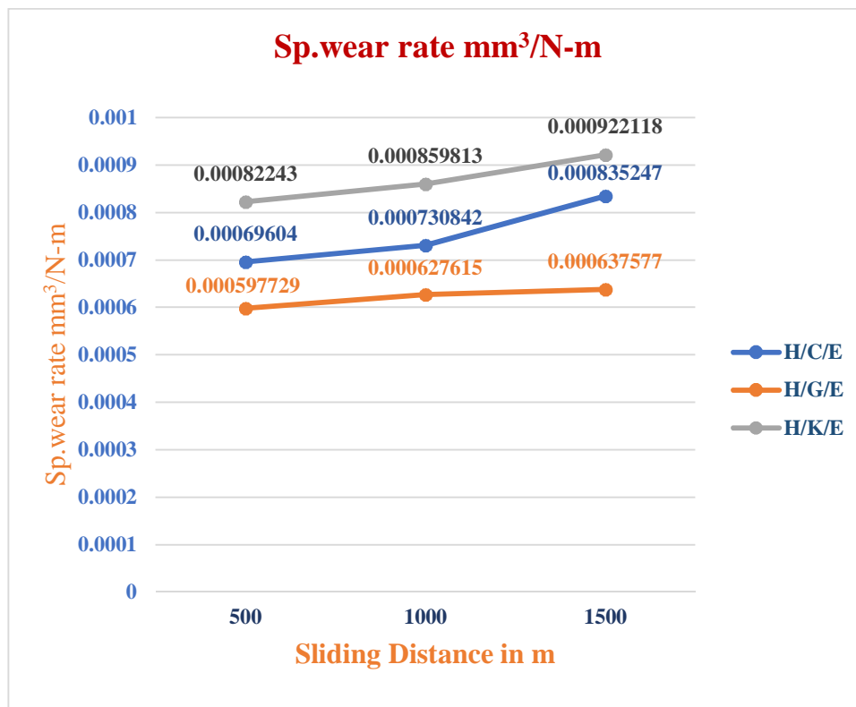
Figure 1(b) Specific Wear rate of Hybrid composites
