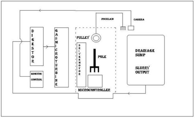
On analyzing the schematic diagram, the output slurry is fed to a digester and sewer gas produced from digester is given as input to run the turbine thus producing a power output; this output power is given to the microcontroller and driver motor thus the hydraulic-pock lain interaction is facilitated and the movement of pock lain is controlled by human control (through system monitor)
