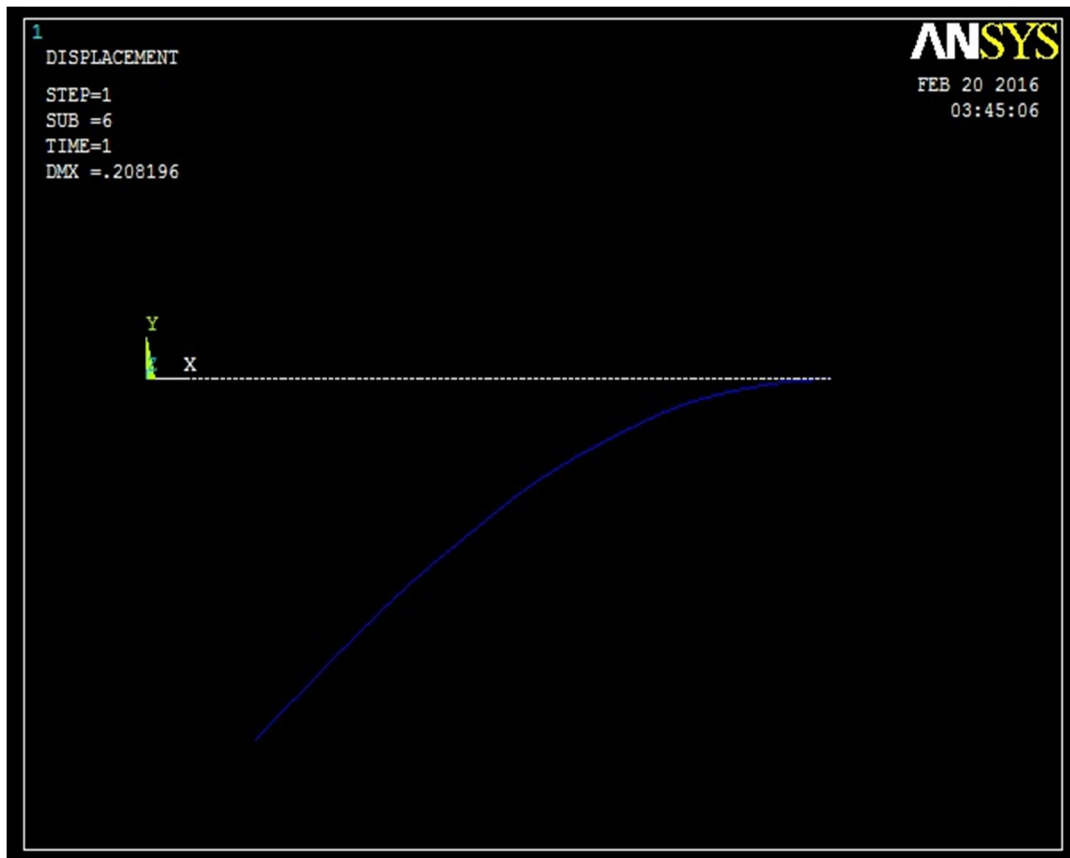
Figure 2: ANSYS deflection when 500gm weights applied
