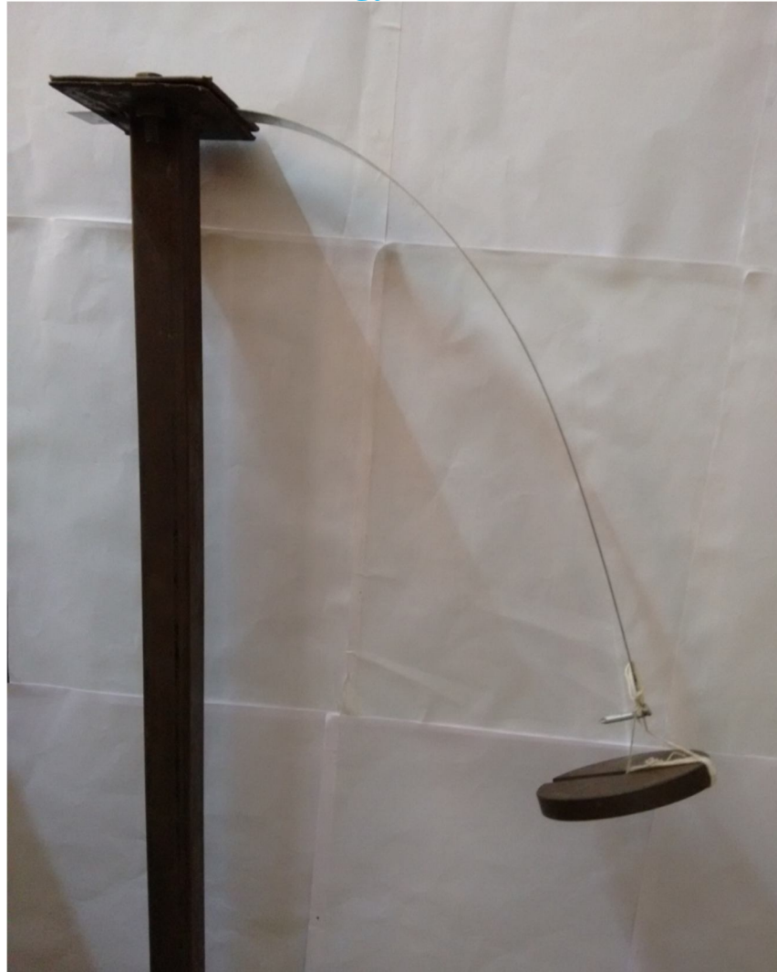
Figure 1: Experimental set-up when 500 gm weights applied.
