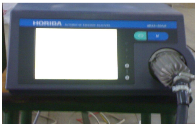
Figure 4 HORIBA Exhaust gas Analyzer
