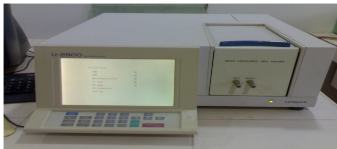
Figure.8(b) Schematic of UV-Spectrophotometer
