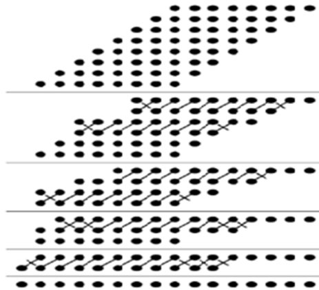
Fig.8. 8 bit conventional Wallace tree
