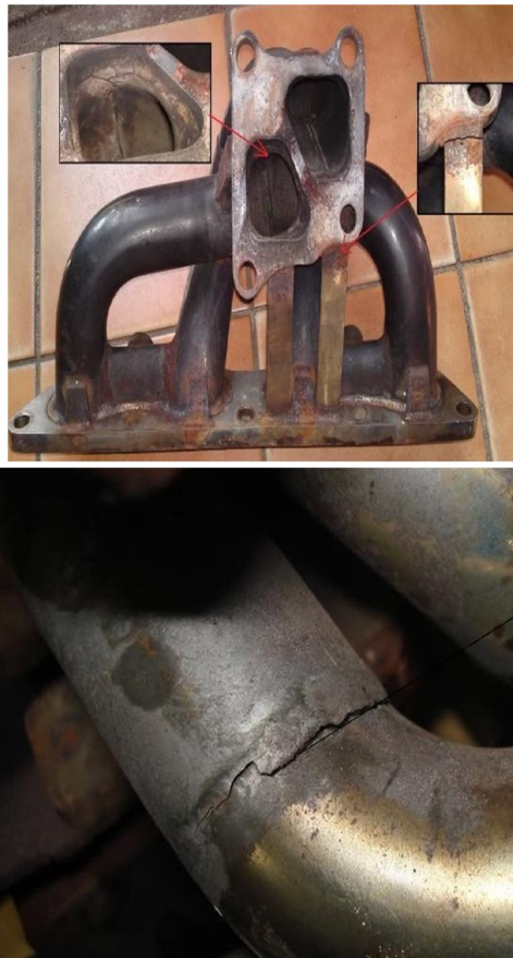
Fig.1. Defects in End connections due to thermal stress
