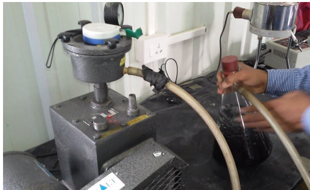
Fig 5: Air Voids determination setup
