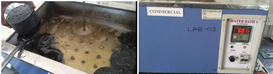
Fig 3: moulds immersed in water bath for 24 hours
