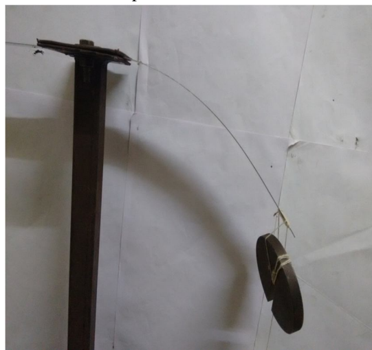
Figure 2: Experimental set-up when length is 0.250m.
