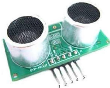
Figure 2: Pin interface of Ultrasonic sensor
