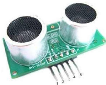
Figure 2: Pin interface of Ultrasonic sensor
