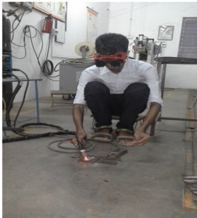
FIG-1:-Indicates joining of two plates by tig welding
