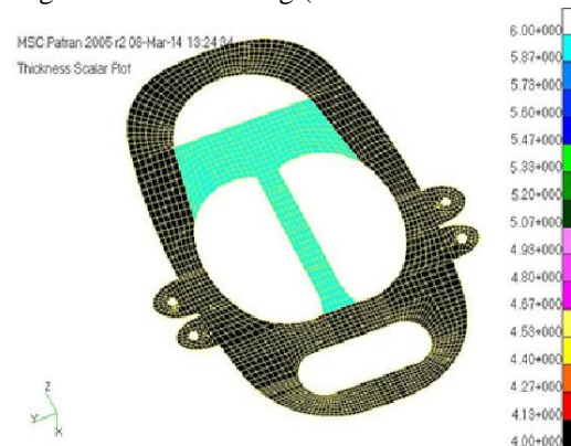
Fig 12: Bulkhead with 4mm and 6mm thickness
