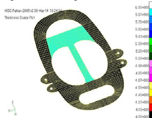
Fig 12: Bulkhead with 4mm and 6mm thickness
