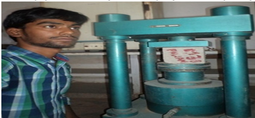
Figure1: Cube testing by compression testing machine
