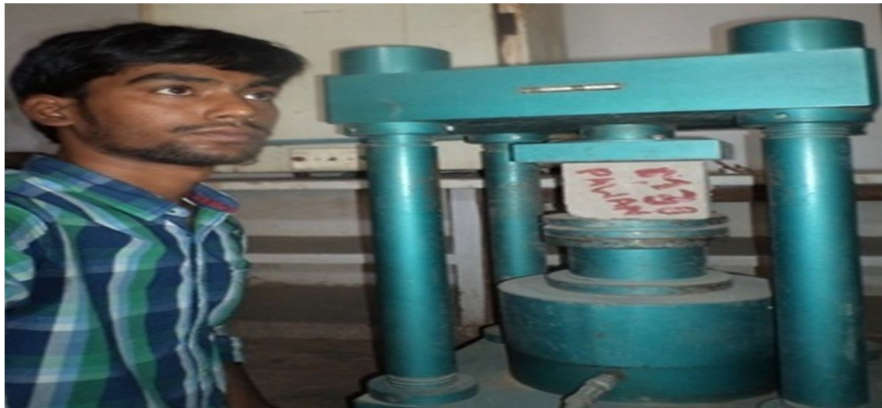
Figure1: Cube testing by compression testing machine
