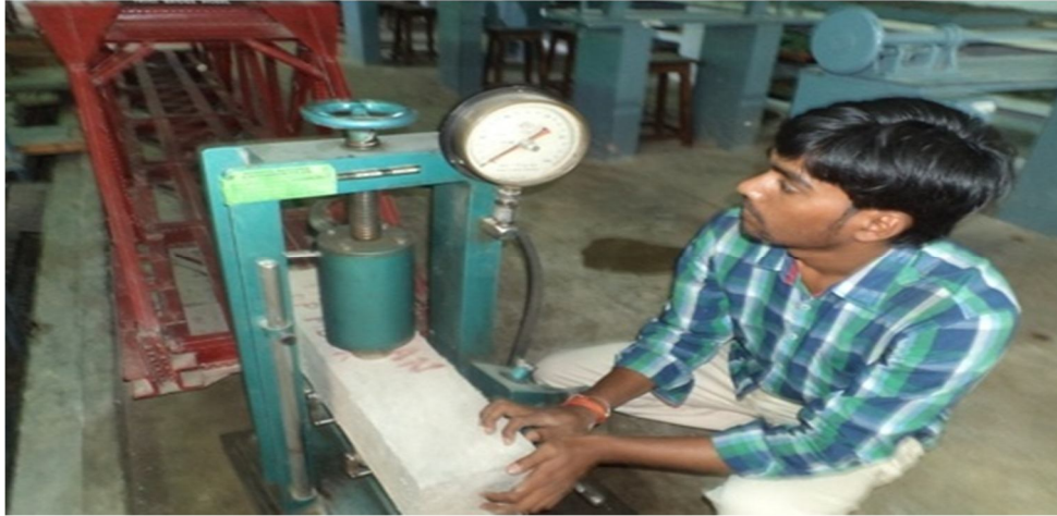
Figure3: Beam testing of manual flexural testing machine
