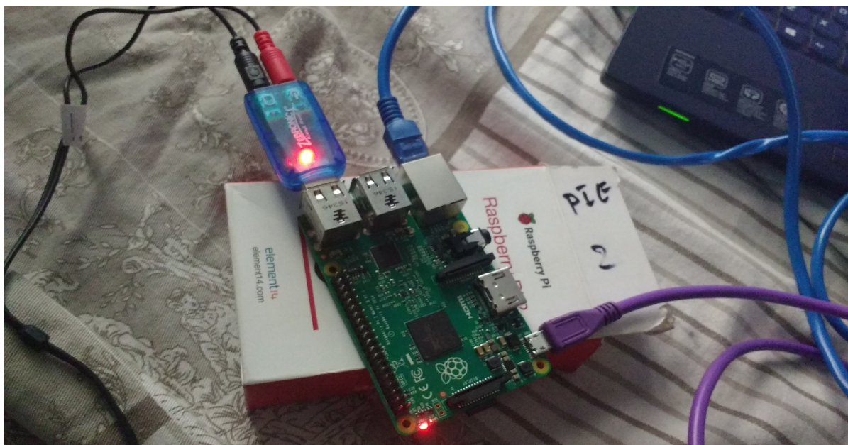
Fig 4.2 voice recognizer unit on Raspberry pi 2 model B
