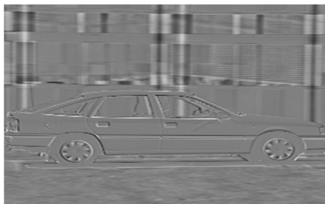
Fig.3 Image showing Frame Difference of block size 2x2
