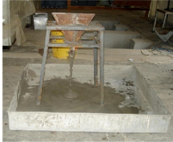
FIG 6: V-FUNNEL TESTS EQUIPMENT
