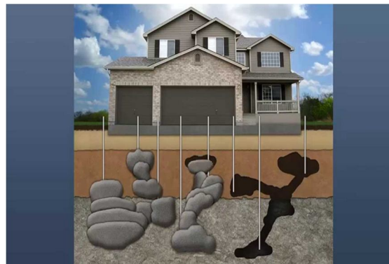
Figure: Compaction grouting
