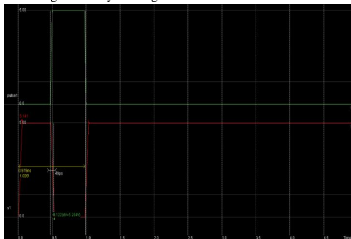
Figure 5: Timing (analog simulation) diagram for the CMOS Inverter
