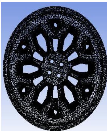
Fig. 4 Meshing of wheel rim
