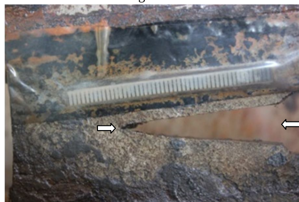
(d). 1,97,962 cycles Crack length: 39.77 mm
