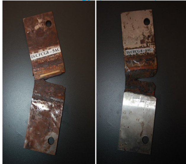
Fig. 5 Close-up view of specimen after failure
