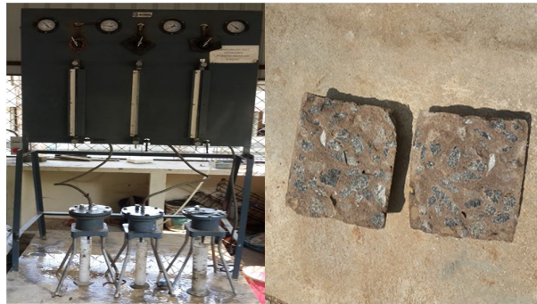
Fig 9. Water permeability apparatus and Tested material
