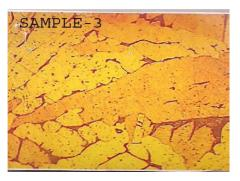
The matrix shows cast fine inter-dendritic grains of alpha and beta. The matrix is beta and the presence of alpha solid solution is about 20% in a matrix of beta solid solution. Void shows the material is cast and due to shrinkage defect
