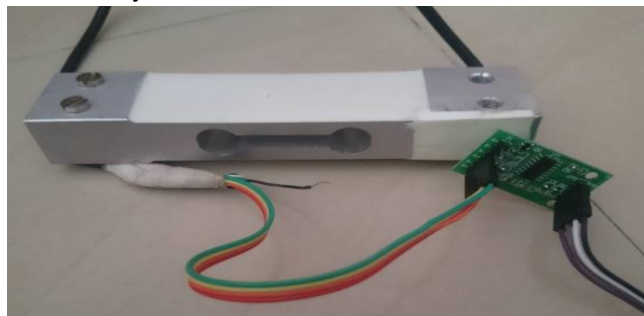
Fig. 4. Strain Gauge Load Cell
