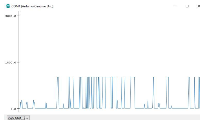
Fig. 13. Sound detector detecting the whistles vs time
