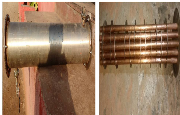
Fig.2: schematic view of Shell and Tube
