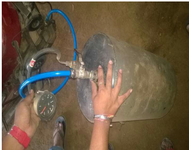
Fig. No.:-6 Pressure Gauge System
