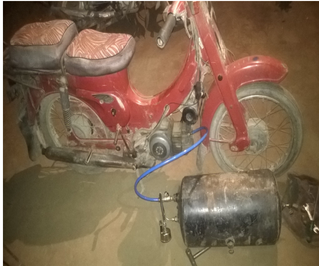
Fig. No.:-3 Working-Compressed air engine
