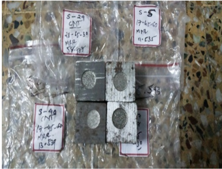
Fig 3 experiment specimen by EDM Machine
