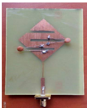
Fig 6. Fabricated three slots with capacitor on radiating patch of RMSA with microstrip line feed
