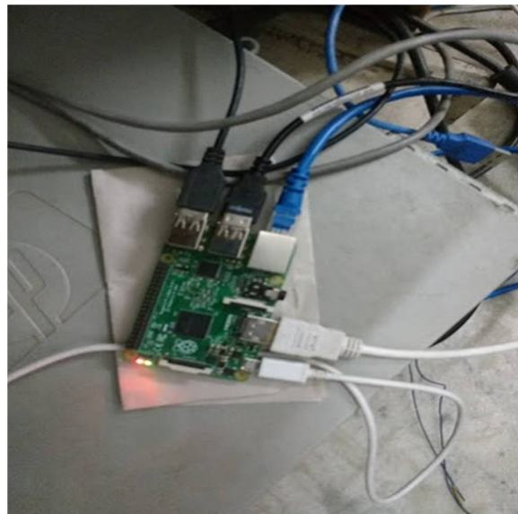
Fig 4: Raspberry Pi Board Connections.
