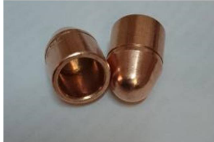
Fig 2: Photograph of Class 2 Copper Chromium electrode.
