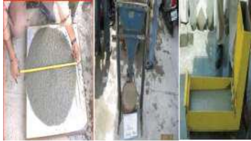
Fig. 1: Slump flow, V-funnel, L-box test
