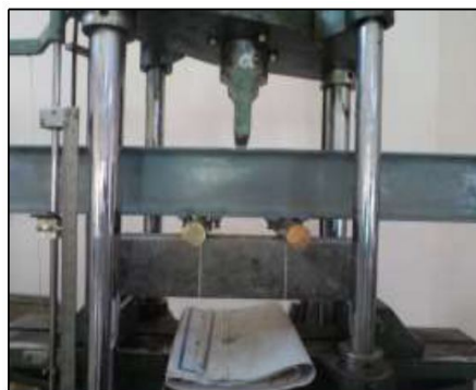
Fig. 4: Flexural Strength Test
