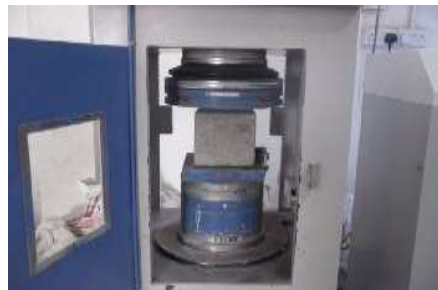
Fig. 2: Compressive Strength Test
