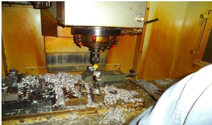
Figure 5.3.6 shows the finished component inspection on machine
