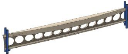
Fig 2. Lateral torsional buckling mode of cellular beams
