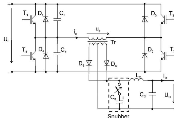
Fig.1: Principle of the ZVZCS PS-PWM converter operation.
